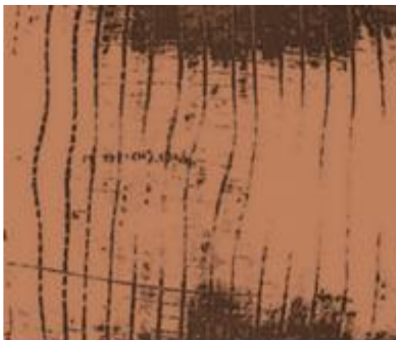
Fig. 8. Intermediate shape of the blank when punching a circle from a strip in case of loss of stability (bend) in the region of the side face, parallel to the axis of the strips.
