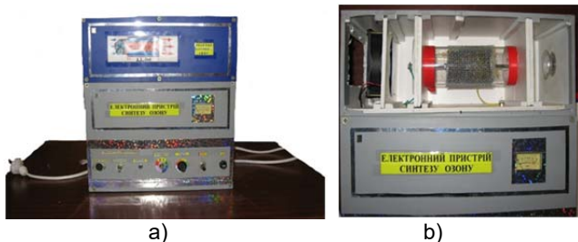
Fig. 2. Electronic ozone synthesis device: a – general form; b – ozone synthesis working chamber.
