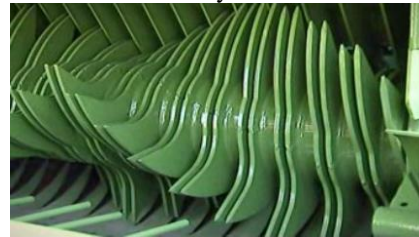
View of the feeding rotor of the Multi Cut baler Round Pack 1250, 1550 by Krone
