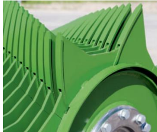
Fig. 7. Location of teeth on AX (25 mm) and MX (17 mm) pick-up trucks by Krone
