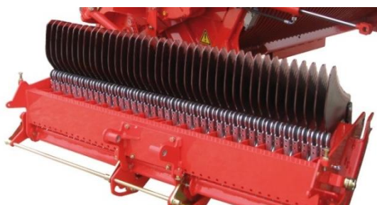
Fig. 5. Torro 5100 LD pick-up truck cutting mechanism by Pottinger
