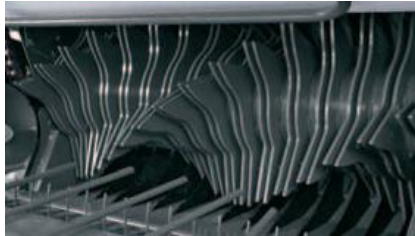
View of the feeding rotor of the Roto Cut baler Variant 380 RC by Claas
