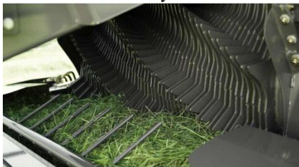
View of the feeding rotor of the Quadrant 3400 RC baler by Claas
