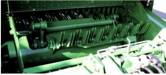
Fig. 2. Scheme of the shredding machine with controlled rakes of Titan pick-up trucks
