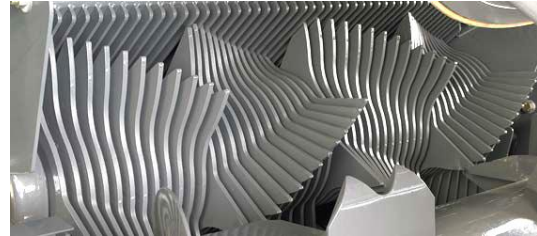
View of the Fine Cut feeder rotor of Quadrant 3200 FC baler by Claas
