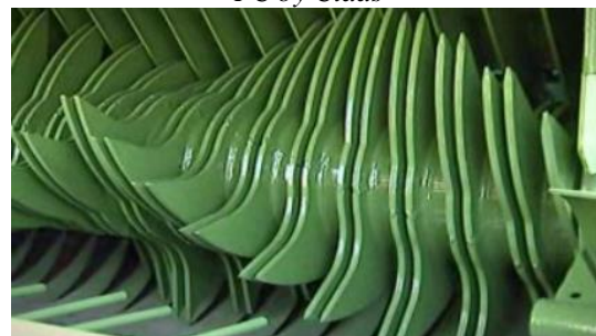
Form of feed rotor Multi Cut baler Round Pack 1250, 1550 by Krone
