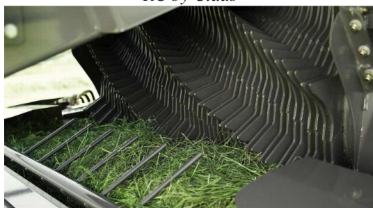
Form of the feed rotor of the baler Quadrant 3400 RC by Claas
