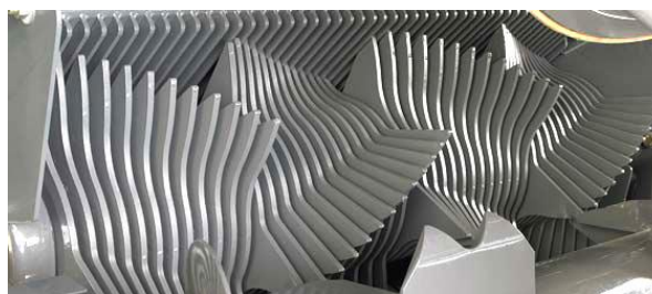
Form of the feed rotor Fine Cut baler Quadrant 3200 FC by Claas
