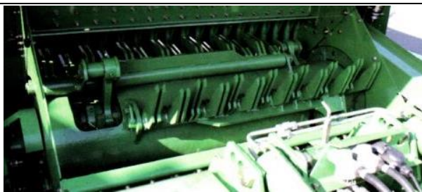
Fig. 6. Scheme of the shredding device with controlled rakes of Titan trolleys
