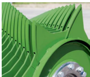
Fig. 12. Location of teeth on AH (25 mm) and MX (17 mm) Krone pick-up truck
