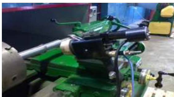
Figure 4. Unit for EAS with a propane-air combustion chamber
