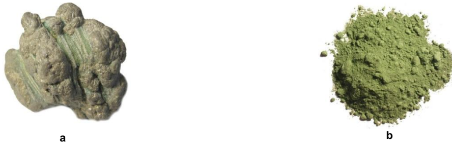
Fig. 3 - glauconite before and after grinding a – glauconite before grinding; b – glauconite after grinding
