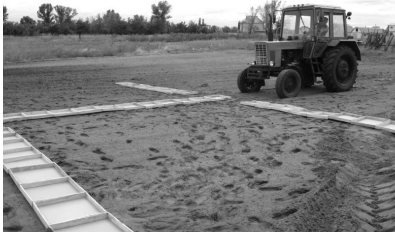
Fig. 1 - Placement of trays on the field to determine the uniformity of fertilizer spreading
