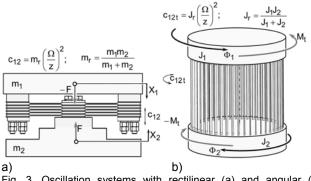
Fig. 3. Oscillation systems with rectilinear (a) and angular (b) movement
