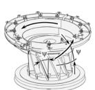
Fig. 1. Vibrating bunker feeders with guided (screw-like) oscillations in which the bowl is made cylinder-like (a) and a conical-like (b)
