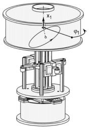
Fig. 2. Vibrating bunker feeder with independent (elliptical) oscillations
