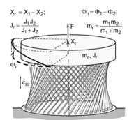
Fig. 5. An oscillation system based on a hyperboloid torsion, reduced to single weight
