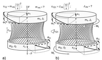
Fig. 4. An oscillation system based on a hyperboloid torsion, driven by the force of disturbance (a) and torque (b), and carries a propeller motion, where  $X_i$  and  $\Phi_i$ , respectively, the amplitudes of bodies in linear and angular oscillations
