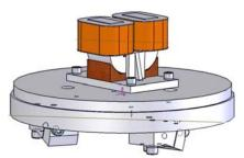
Fig. 8. The reactive mass, the mass of which is  $m_2 = 34.4 \text{ kg}$ , and the moment of inertia relative to the axis of rotation  $J_2 = 0.37 \text{ kg} \cdot \text{m}^2$
