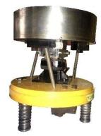
Fig. 9. Photo of a vibrating bunker feeder
