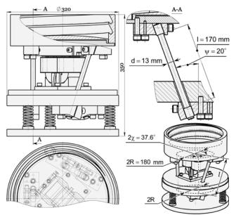
Fig. 6. General view of the vibration bunker Fedder
