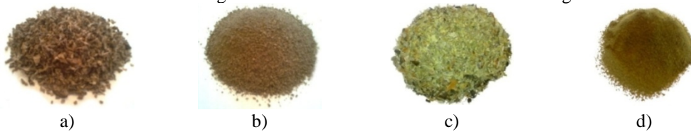
Fig. 10. Material before and after grinding: a, b – roots of valerianum before and after crushing; c, d – collecting herbs before and after grinding
