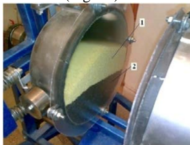
Fig. 14. Distribution of parts of treated material when loading: 1 – millet; 2 – rape
